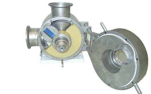
Please note that the weight of the front cover is about 140 pound. When any parts inside the pump have to be replaced or the pump itself must be cleaned inside, it is necessary to take off the front cover.
