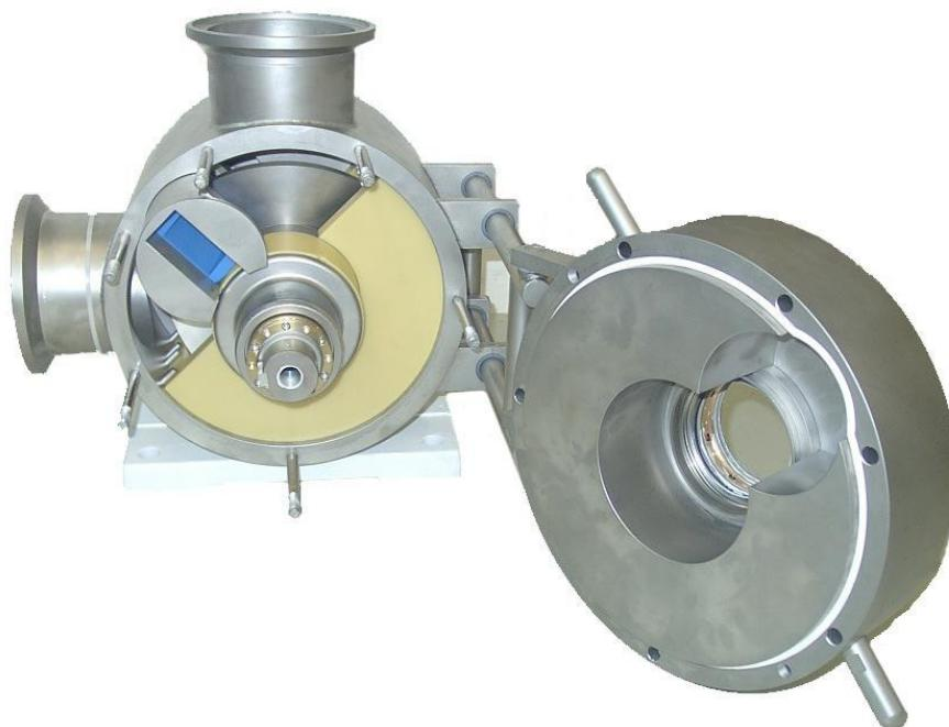
Please note that the weight of the front cover is about 140 pound. When any parts inside the pump have to be replaced or the pump itself must be cleaned inside, it is necessary to take off the front cover.
